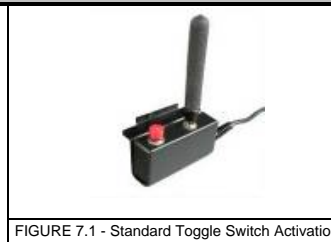
FIGURE 7.1 - Standard Toggle Switch Activation
