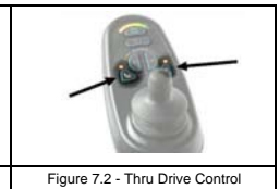
Figure 7.2 - Thru Drive Control
